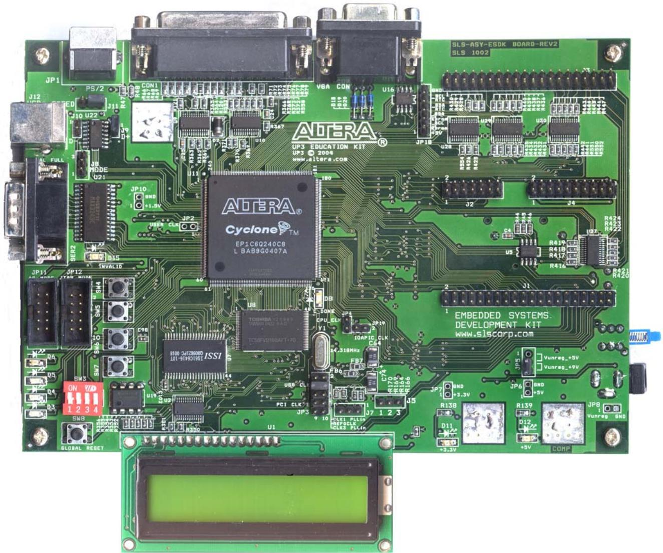
**Figure 1.1** The Altera UP 3 FPGA Development board
