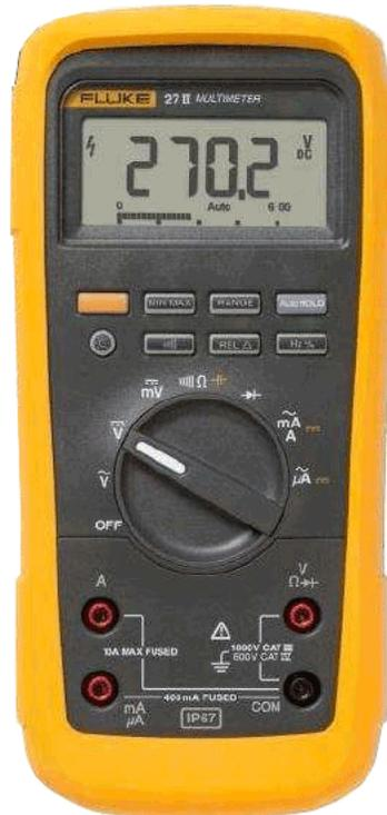
A Fluke Digital Multimeter
