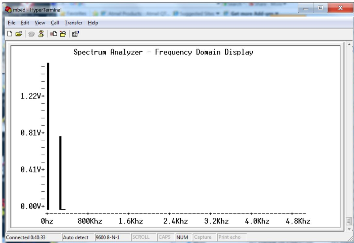
VT100 Spectrum Analyzer display using the sine wave input signal
