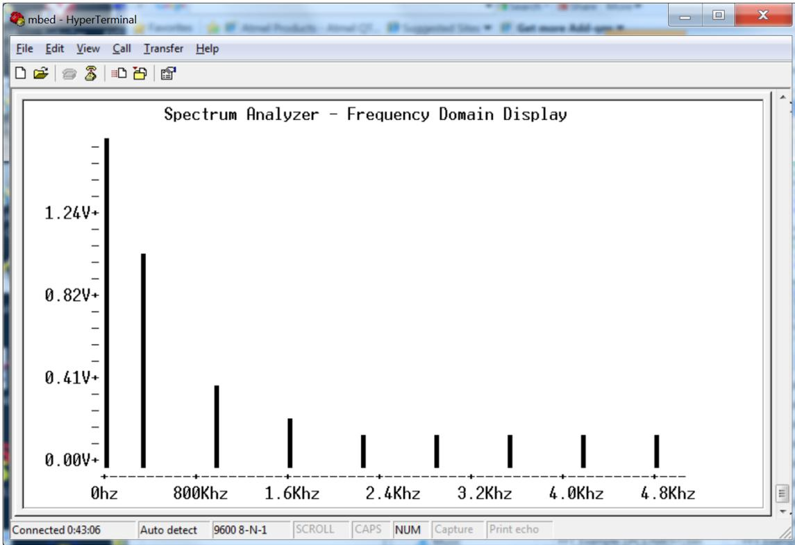
VT100 Spectrum Analyzer display using the square wave input signal.
