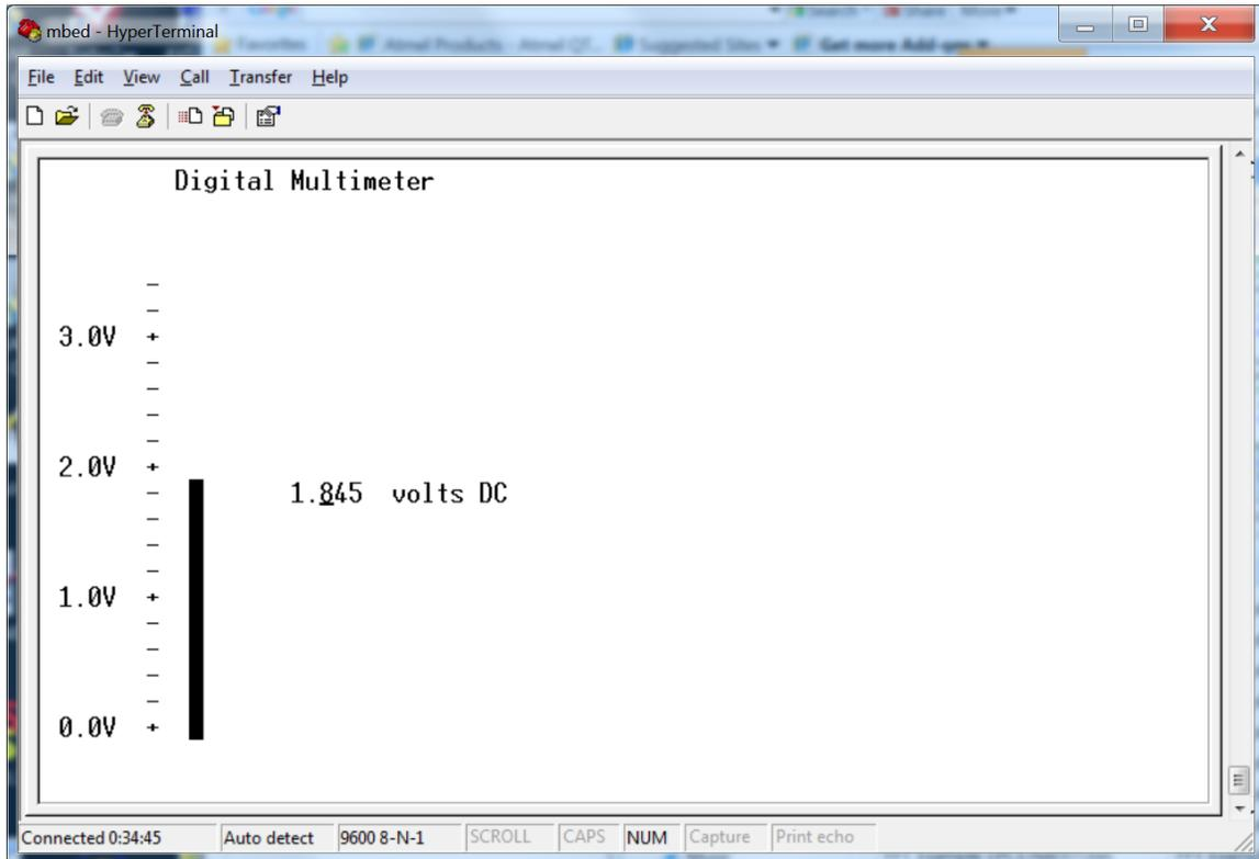
VT100 DMM display with an analog input signal generated by the D/A
