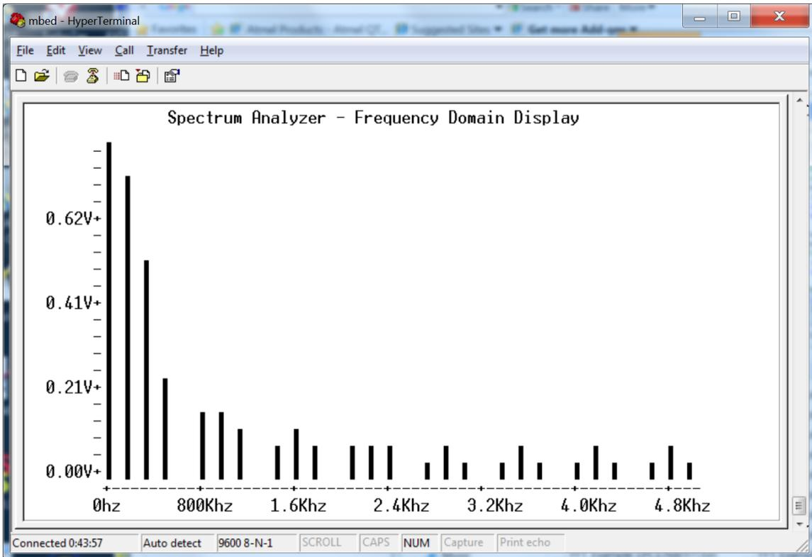
VT100 Spectrum Analyzer using the square wave input signal with a 25% duty cycle.
