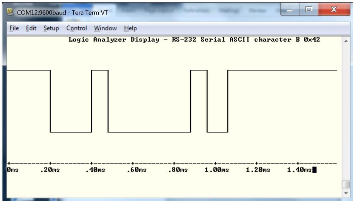
The VT100 Logic Analyzer Display for a character sent out as a serial bit stream.
