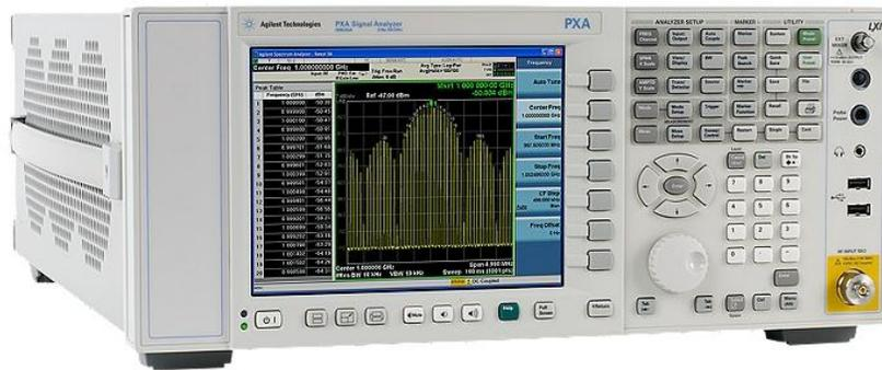
An Agilent Spectrum Analyzer displaying the frequency content of a signal
