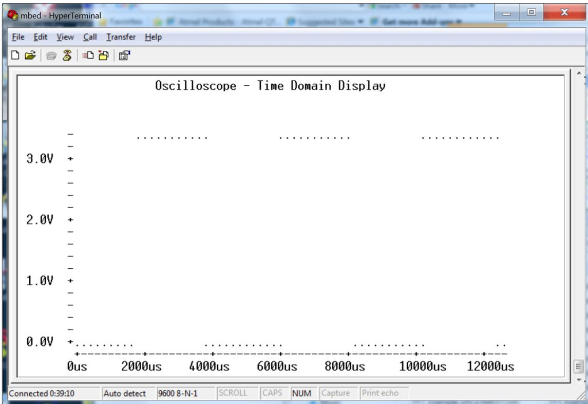
VT100 Oscilloscope display using square wave generated by PWM hardware.
