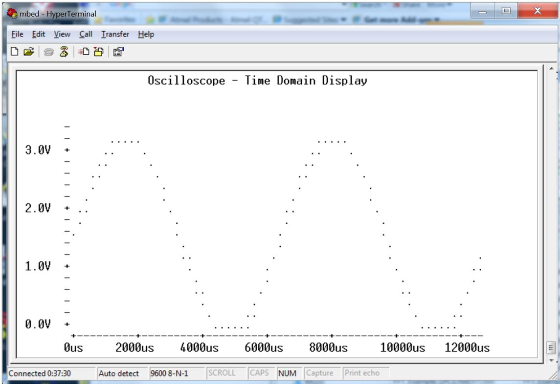
VT100 Oscilloscope display using sine wave source generated by D/A
